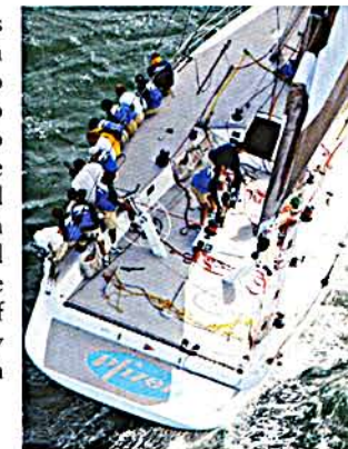
Subtle stern treatment - not very. Cometa is wide and powerful and relies on a huge rig and a leeward-canted keel in light air
